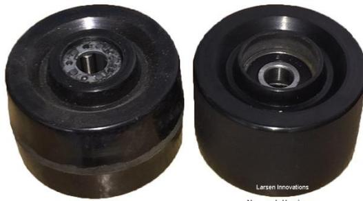
New - sealed bearings on bottom guide rollers
