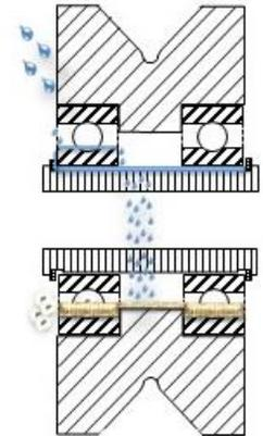
Competitor's roller uses a shielded NOT sealed bearing which permits moisture and dust to enter
