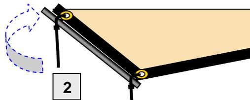
Fasten the vinyl roof tarp loosely at each point then tighten the ties to evenly space the tarp on the roof truss assembly. Cut off the excess tie material for a clean look. Use **CARE** not to leave a sharp pointed end on the tie when cutting.
