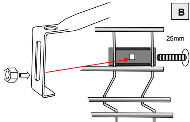
**(B) OPTIONAL** – you may mount the third truss in the center of the 6' panels as shown. **This will require that you cut each of the two ridgeline braces to fit.**
